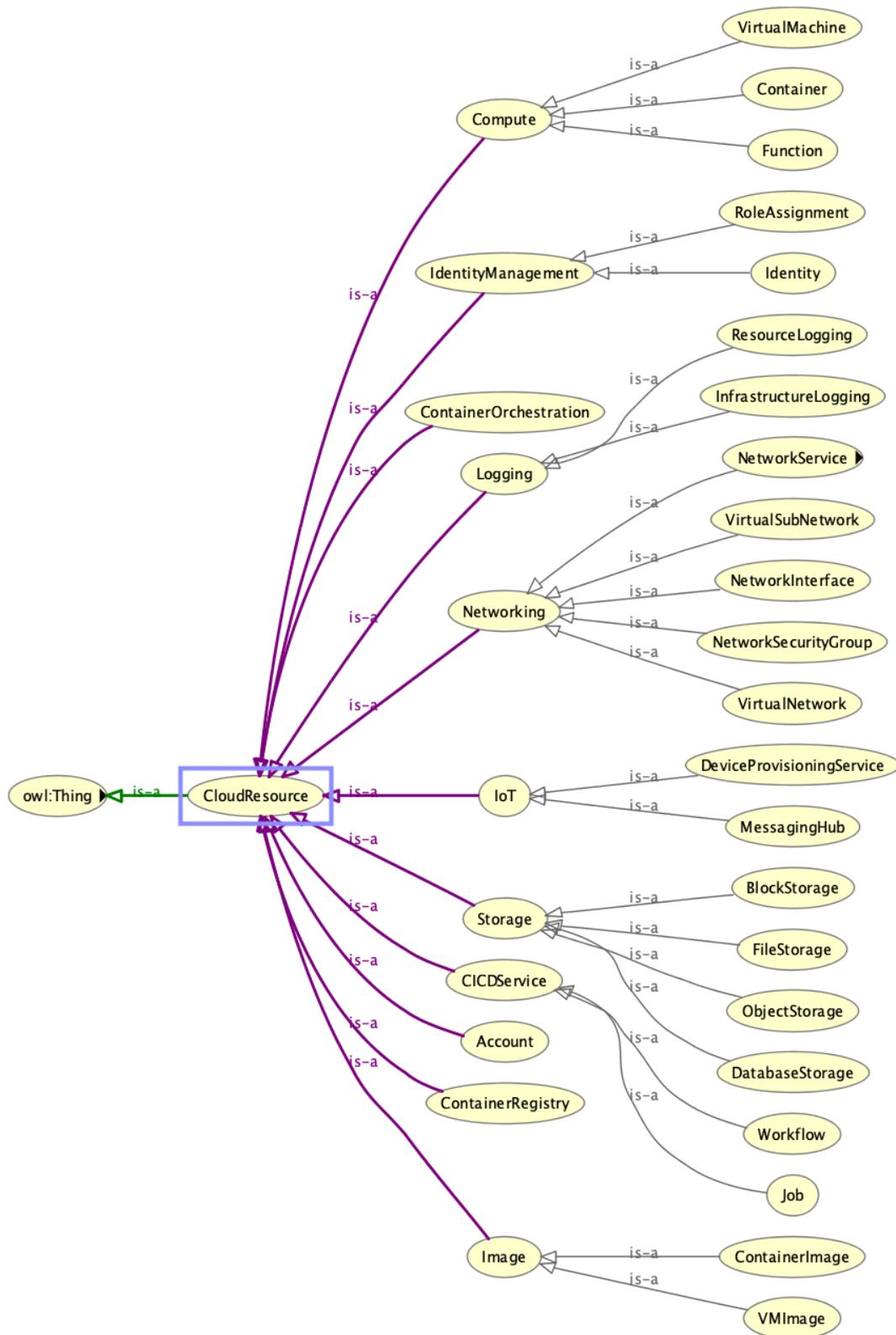
Figure 31. The cloud resource taxonomy which classifies cloud resources according to their functional purpose, like compute, storage, and networking
