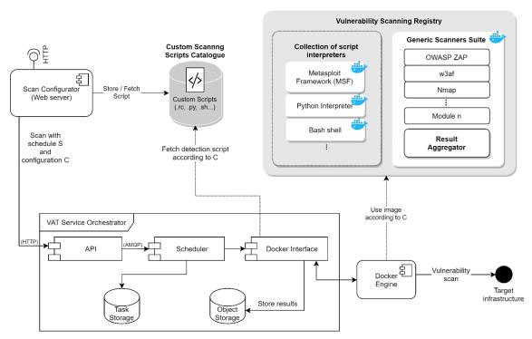
Figure 8. Internal architecture schema of Vulnerability Assessment Tools
