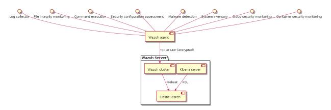
Figure 6. High-level Wazuh's architecture
