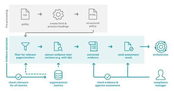
Figure 11. Main architecture for AMOE (keyword-based extraction method)
