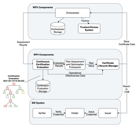
Figure 3. Overall Architecture of WP4 components and connection to WP3 components (source: MEDINA's own contribution)
